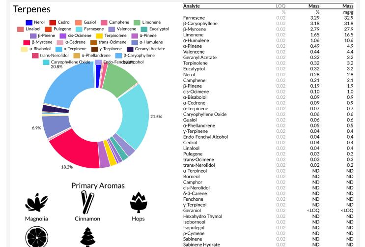
Date Tested: 06/22/2021; Analysis performed on Agilent 7890A GCFID
