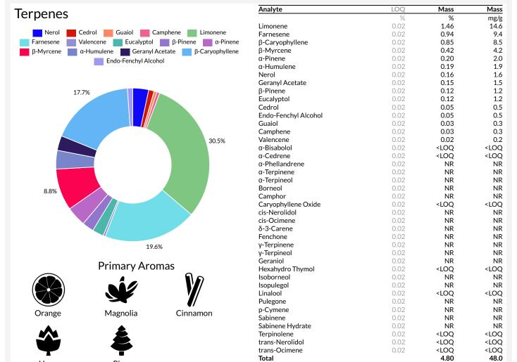
Date Tested: 02/10/2021; Analysis performed on Agilent 7890A GCFID
