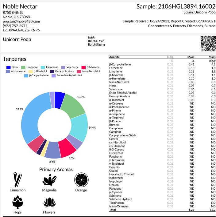
Date Tested: 06/28/2021; Analysis performed on Agilent 7890A GCFID
